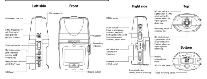
The Zoom H2n is capable of recording very high quality audio in a range of stereo and surround polar patterns. You can control the recording pattern using the switch on the top of the unit. Here are the basic operation instructions:
